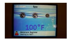
After you exit the programming mode your hot tub will automatically heat to the factory preset default temperature of 38°C (100°F).
