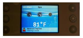
The keypad does not store the date and time so when the system starts up after a loss of power a message will prompt you to reprogram the time and date.
