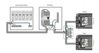
230 VOLT DUAL PHASE RCD WIRING
