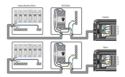
230 VOLT THREE PHASE RCD WIRING
