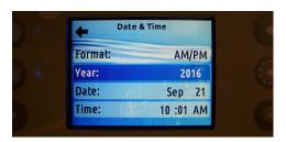
Here you can adjust the time format (AM/PM or 24h), day of the week and time. Use the arrows to choose the setting that you want to adjust and select it by pressing the Light key. Use the arrow buttons to change the parameters and the Light key to move between parameters. Pump 1 will take you back to the main Settings menu.
