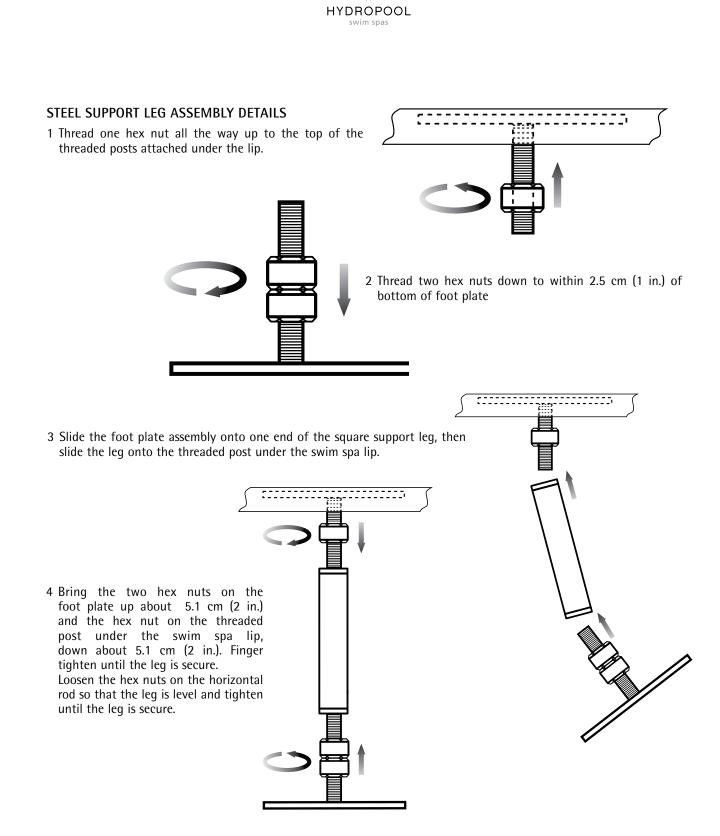
5 After the swim spa is filled with water, the legs can now be adjusted as necessary from either the top or bottom with a wrench to ensure that the walls are straight and level. See section FILLING, CHECKING & STARTING YOUR SWIM SPA
