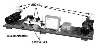
RELEASING AIR TRAPPED IN FILTER...
