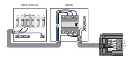
230 VOLT THREE PHASE RCD WIRING (IN.XM PACK ONLY)
