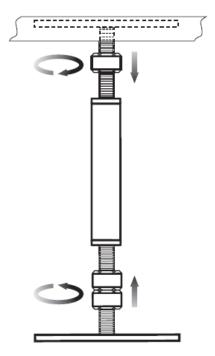
4 Bring the two hex nuts on the foot plate up about 5.1 cm (2 in.) and the hex nut on the threaded post under the swim spa lip, down about 5.1 cm (2 in.). Finger tighten until the leg is secure. Loosen the hex nuts on the horizontal rod so that the leg is level and tighten until the leg is secure.
