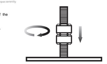
2 Thread two hex nuts down to within 2.5 cm (1 in.) of bottom of foot plate
