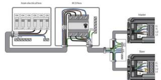
230 VOLT THREE PHASE RCD WIRING
