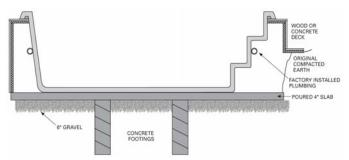
• It is recommended leaving a 61 cm (24 in) wide crawl-space around the entire unit to ensure adequate accessibility.
