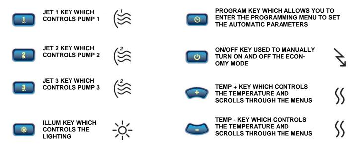
Use the (+) or (-) keys to set desired water temperature or raise or lower values in a menu. Use the (<) or (>) keys to move between selections.
