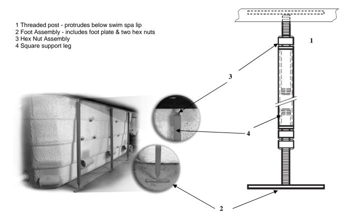
**1** Thread one hex nut all the way up to the top of the threaded posts attached under the lip.
