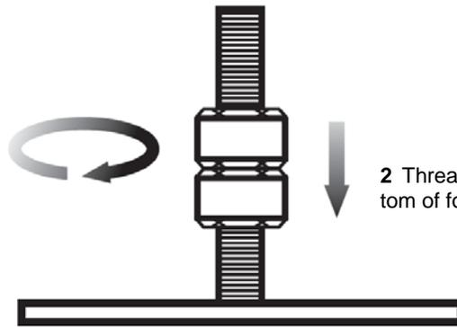
2 Thread two hex nuts down to within 2.5 cm (1 in.) of bottom of foot plate
