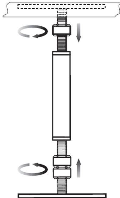
5 After the swim spa is filled with water, the legs can now be adjusted as necessary from either the top or bottom with a wrench to ensure that the walls are straight and level. See section **FILLING, CHECKING & STARTING YOUR SWIM SPA**
