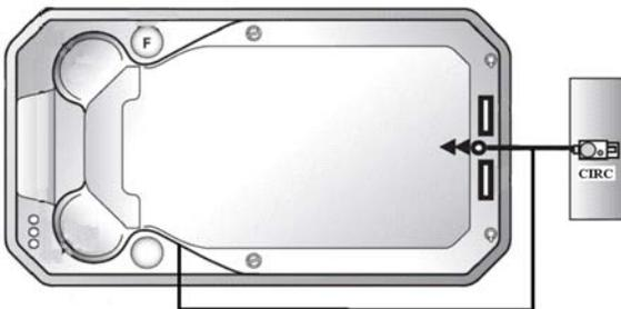
Inlet/Suction Side Plumbing Connections
