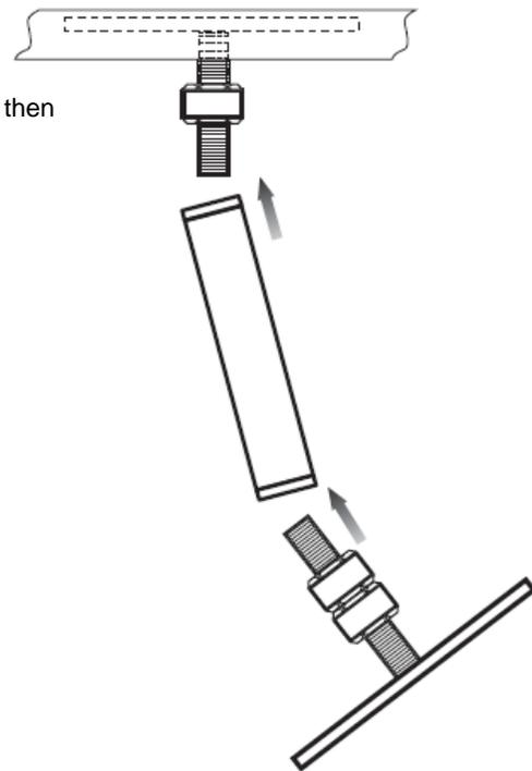
4 Bring the two hex nuts on the foot plate up about 5.1 cm (2 in.) and the hex nut on the threaded post under the swim spa lip, down about 5.1 cm (2 in.). Finger tighten until the leg is secure. Loosen the hex nuts on the horizontal rod so that the leg is level and tighten until the leg is secure.
