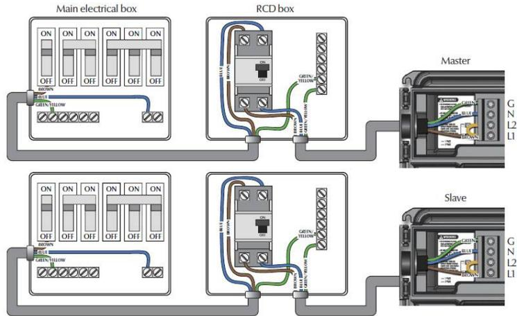
**230 VOLT THREE PHASE RCD WIRING**
