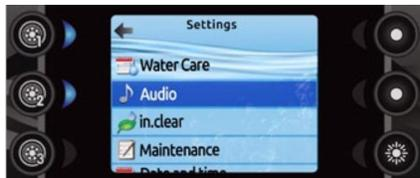
Use the arrow keys to move up and down in the list. To select an option, press the lit button beside it (Light button).
