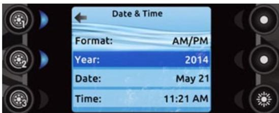
Here you can adjust the time format (AM/PM or 24h), day of the week and time. Use the arrows to choose the setting that you want to adjust and select it by pressing the Light key. Use the arrow buttons to change the parameters and the Light key to move between parameters. Pump 1 will take you back to the main Settings menu.
