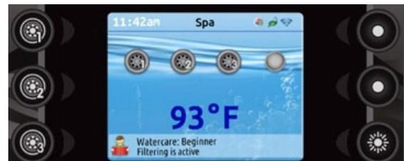
After you exit the programming mode your hot tub will automatically heat to the factory preset default temperature of 38°C (100°F).
