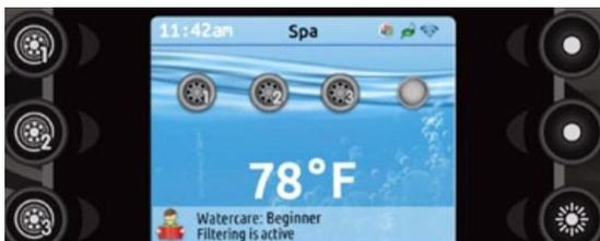
The keypad does not store the date and time so when the system starts up after a loss of power a message will prompt you to reprogram the time and date.
