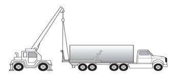
Most Hydropool models require a clearance width of at least 100 cm. (39 in.) to allow movement of the unit on its side through alley-ways, fence openings, etc. Where this is not possible, the use of a crane to lift the hot tub from the truck or trailer over the house to the patio or yard is often a simple and economical option.
