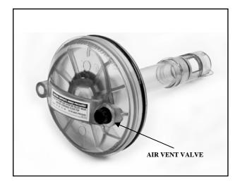
• When the pump starts circulating, it will be necessary to release trapped air in the filter. Carefully loosen the air vent valve counter-clockwise until there is the hissing sound of air escaping. Once there is a steady stream of water, close the vent valve, ensuring that the o-ring does not become pinched.
