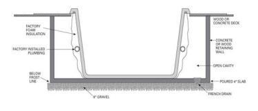
• Non-freezing climates – it is sufficient to ensure that the base of the hole or cavity created for the tub has a dry, stable, compacted level base and proper drainage
